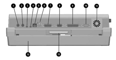
Figure 1-6. Expansion Base Components - Rear Panel (MultiBay-ISA Illustrated)
